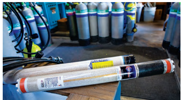
Correctly designed filters should remove the standard contaminants found in compressed air.
